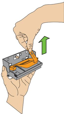
**c)** Pull on the orange tab to remove the protective retainer.
